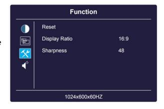
Sharpness: Adjust the picture sharpness. The adjusting range is from 0 to 100.
